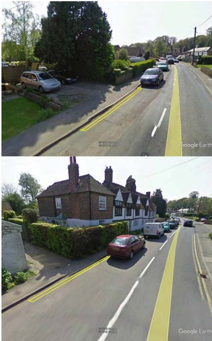
Figure 7: Indicative illustration of proposed double yellow lines across driveways to formalise passing bays
