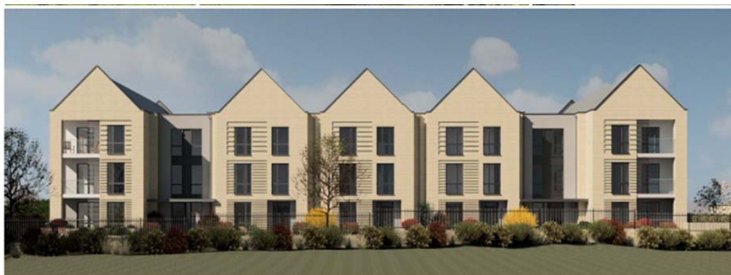
Figure 10: CGI rendering of north-east elevation facing green space scheme showing projecting brickwork and circulation cores
